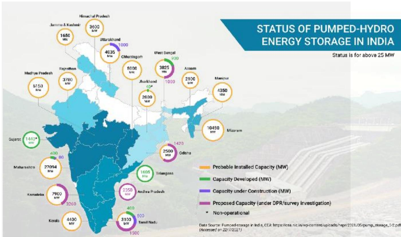
Though India has tremendous potential for PHES, only six plants with a total of 3305.06 MW are currently under operational capacity in four states. However, of these, three plants with a cumulative capacity of 1480 MW are currently not operational in pumping mode due to the following issues:
